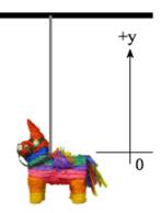
$$\omega = \sqrt{\frac{k}{m}} = \sqrt{\frac{40N/m}{2 \, kg}} = \sqrt{20 \, \frac{1}{s^2}} = 4.47 \, \frac{\text{rad}}{\text{s}}; f = \frac{\omega}{2\pi} = \frac{4.47 \, \text{rad/s}}{2\pi \, \text{rad}} = 0.712 \, \text{Hz};$$
