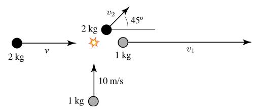
Objects 1 and 2 (with masses 1.0 and 2.0 kg), collide *perfectly elastically* at right angles. The 1 kg object is deflected by 90°; the 2 kg object is deflected by 45°. Object 1 enters with a speed of 10 m/s.
